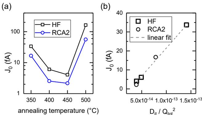
Fig. 3 (a) J<sub>0</sub> of Al<sub>2</sub>O<sub>3</sub> films on p-type c-Si as a function of annealing temperature (b) J<sub>0</sub> as a function of D<sub>it</sub> / Q<sub>tot</sub><sup>2</sup>.
