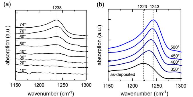
Fig. 2 (a) FTIR absorption spectra of PE-ALD  $\text{AlO}_x$  annealed at 400 °C for various incident angle. (b) Evolution of  $\text{SiO}_x$  LO mode peak at annealing temperature of 350 to 500 °C.
